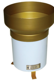
Tipping Bucket with Normally-Open Style Reed Switch Output
